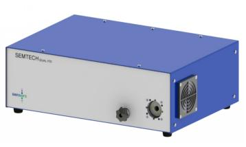
The system is designed to minimize the loss of hydrocarbons prior to analysis by maintaining the required temperature through the use of a heated filter, heated sample line and stainless steel fittings, all of which have low hydrocarbon adsorption characteristics. User-selectable measurement ranges ensure accuracy for a wide variety of test applications.
